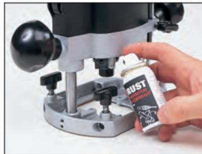
Rustbuster® is used to lubricate the pillars of the router & to prevent surface corrosion.
